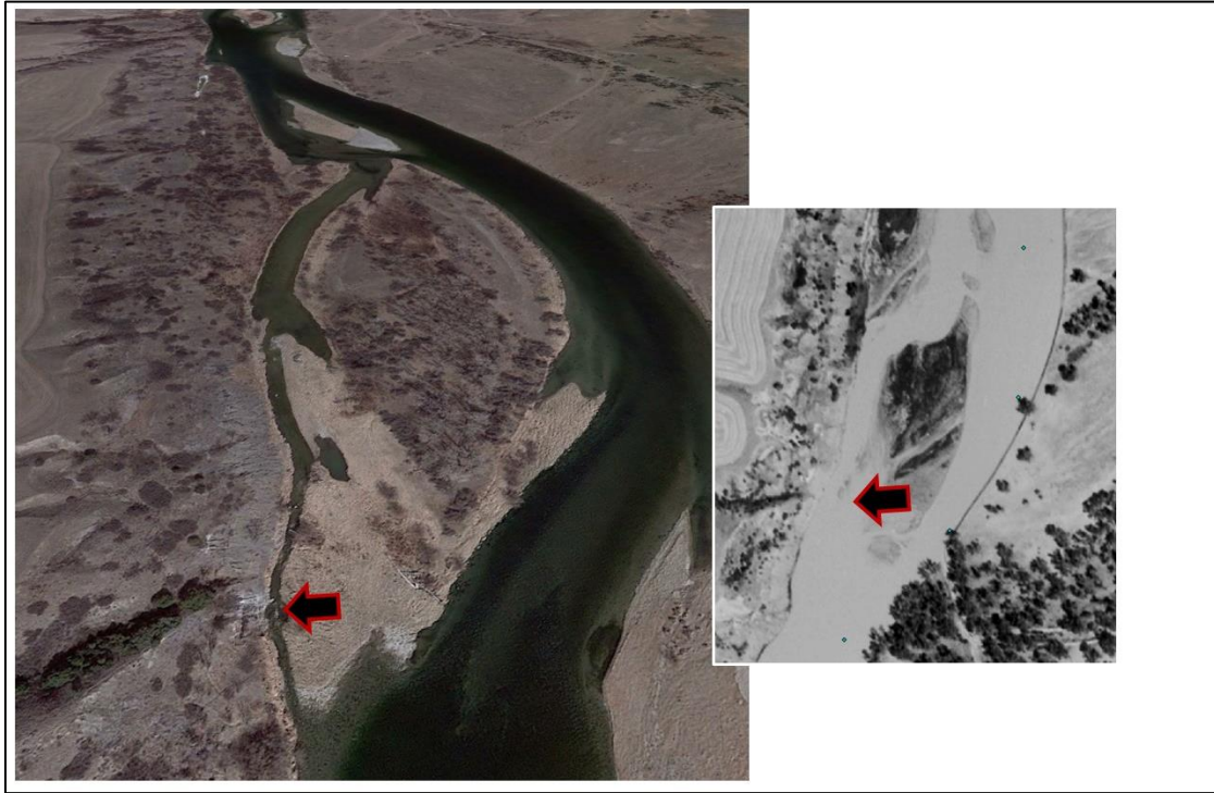
Figure 37. Google Earth Image (2016) showing decaying side channel entrance at RM 64.4; inset shows channel in 1954.
