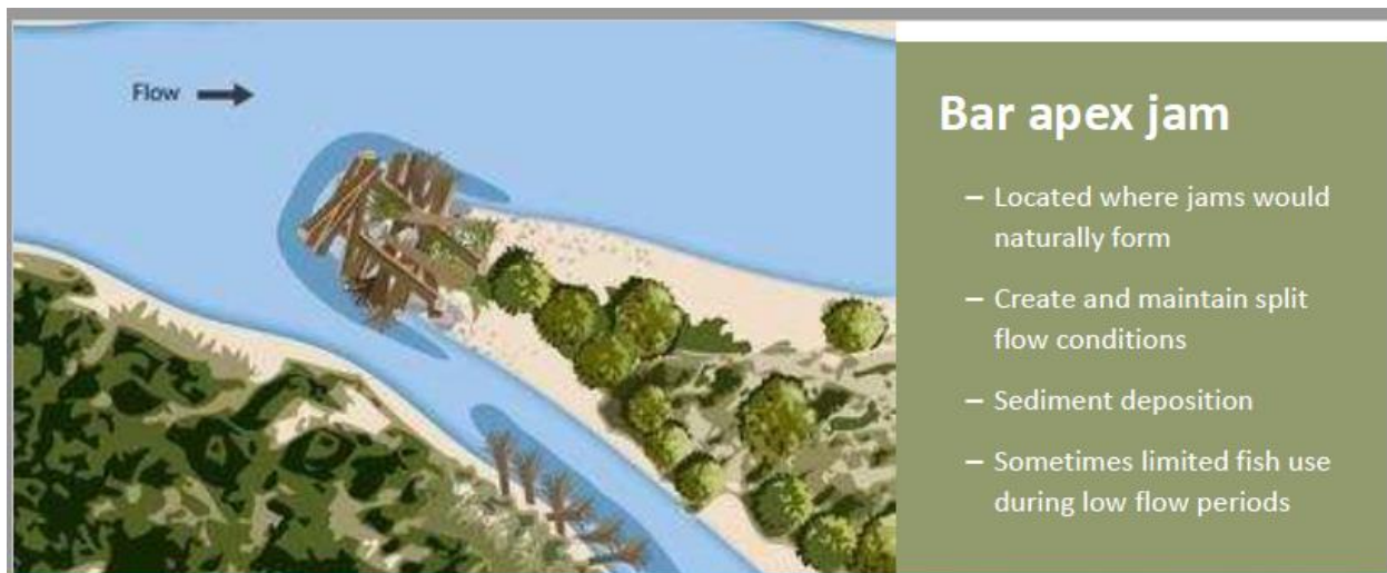
Figure 53. Schematic example of a bar apex jam designed to maintain split flow conditions (Alcott, 2016).
