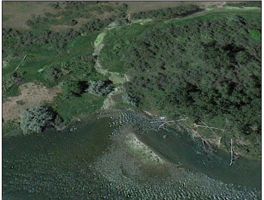
Figure 54. View downs side channel at RM 63.3 showing potential to route additional flows with excavation and/or bar reshaping.
