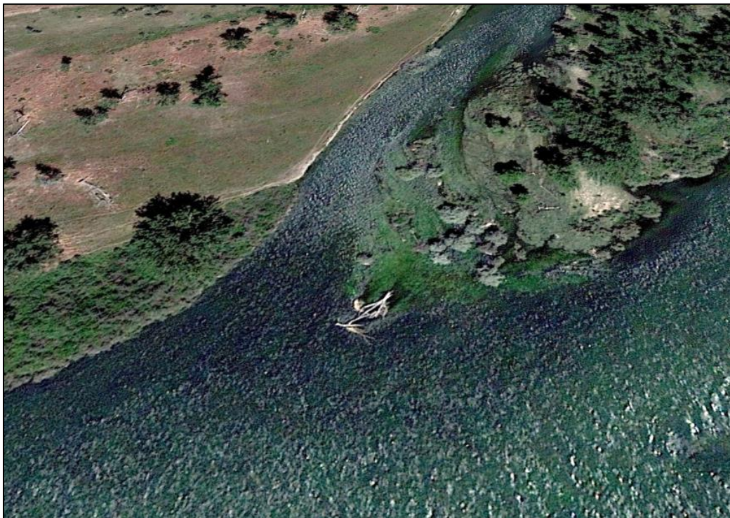
Figure 27. Debris jam at Picture Channel flow split showing how feature facilitates side channel flow.
