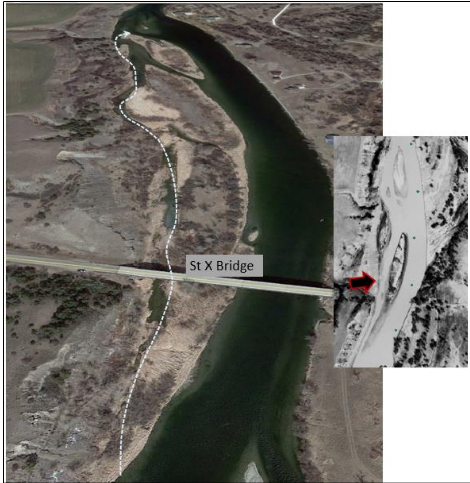
Figure 35. Google Earth Image (2016) disconnected side channel at RM 67.9; inset shows channel in 1954.
