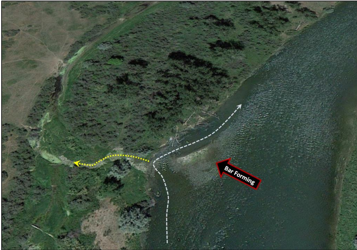
Figure 40. Entrance to channel at RM 63.3 showing bar formation at entrance—channel was not flowing when this image was taken in July 2013.
