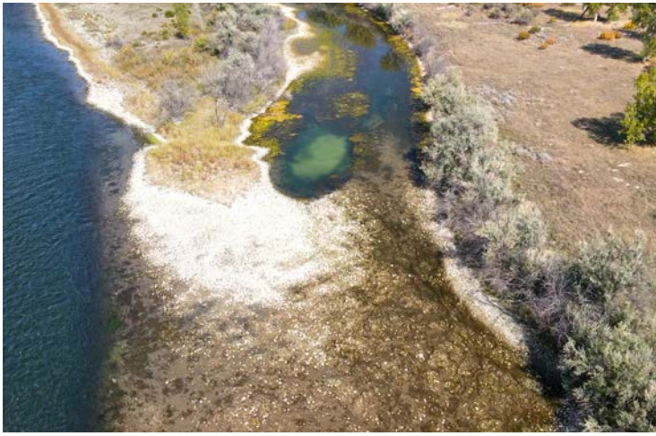
Photo 5. Example of wide, shallow entrance to “Across from Turtle Rock” side channel at 1916 cfs (pre-construction).
